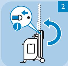
**2** Undo the locking strap **J** and unfold the ironing board to vertical position.
