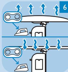
**6** If you want to iron in the blowing mode, press the rounded side of the blowing/suction button. If you want to iron in the suction mode, press the hollow side of the blowing/suction button.
