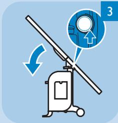
**3** Push the board tilting button **H** and tilt the board to horizontal position.
