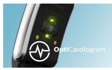
Monitor your heart rate and heart rate zones in real time. The Opticardiogram clinically validated sensing technology tracks Heart Rate (HR), HR Zones, Resting HR and HR Recovery.
