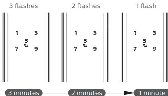
If any of the verification methods among fingerprint, password, or card/key tag has scanned to be incorrect and the number of consecutive incorrect entries reaches 5 times within 5 minutes, the EasyKey will be locked for 3 minutes.
