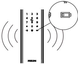
**Triggering:** After waking up, the system will run an automatic examination on the battery voltage. If the voltage is too low, the lock will give an alarm with a voice prompt of “Low battery voltage. Please replace all batteries”.
