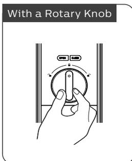
Philips EasyKey employs indoor fast opening mortise. You can unlock from inside by rotating the rotary knob.
