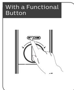
Double press the [OPEN/CLOSE] functional button within one second, then push or pull to unlock.
