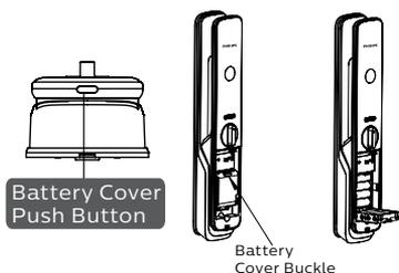
The lock is powered by four 1.5V alkaline batteries. There are two sets of working power stations in the battery cabinet. Eight batteries can put in to extend battery life and reduce battery replacement frequency.
