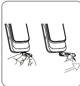
② Insert the key into the keyhole and keep the key and key shell vertical to each other. Rotate the key shell towards the handle for 90° until it closes to the door surface.
