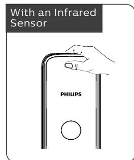
Features with an infrared sensor on the handle, when the sensor is triggered, hold the handle's sensor modules on both the front and rear side simultaneously, you could easily unlock the door.
