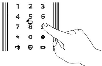
② Press [#] before inputting any other numbers. After hearing a voice prompt of "Enter master PIN code", enter your master PIN code and confirm with [#]. Then you are in master mode.
