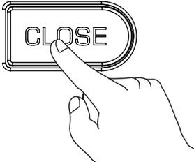
When the EasyKey is locked, long-press the [CLOSE] button, after the indicator flashes once in red, and there will be a voice prompt of "Inside deadlock enabled".
