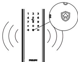
**Triggering:** If the lock is under outside forced lock mode, unlocking from inside will trigger the alarm.
