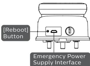
When the battery voltage is insufficient, and the door cannot be opened from the outside, you can power up the lock through the Micro USB interface by using a 5V power bank as an emergency power supply. After opening the door, please replace the batteries immediately.
