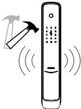
**Triggering 1:** The door is pried open and the sensor latch bolt pops up.
