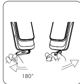
③ Rotate the key shell downwards for 180° to make it parallel to the ground. Then rotate it horizontally towards the handle to unlock the door.
