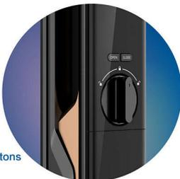
[Open]: Double click the button within one second could unlock the door, which prevents accidentally unlocking by children and pets effectively. [Close]: Click once on the button could lock the door. Long pressing the button could enable inside deadlock. You could use the master PIN code or mechanical key to
