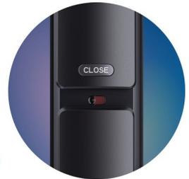
You can enable the safe handle function before you leave home. After the door is locked, the indoor handle will be fixed to ensure that nobody could open the door by pushing the indoor handle. This feature can effectively prevent unlocking from indoor, thus eliminating security risks and improves anti-theft performance.
