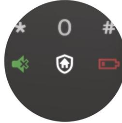
Before leaving home, you can touch the outside forced lock button to enable the function. In this mode, opening the door from inside will trigger an alert. This feature can effectively remind you of security risks and upgrade the level of home security.
