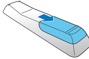
2 Insert 2 AAA batteries with correct polarity (+/-) as indicated.
