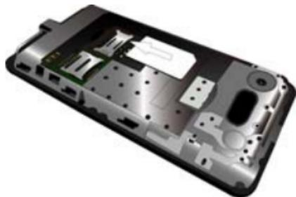
4. As shown, align the metallic connectors on the battery and battery slot. Press the battery down until it is locked.
