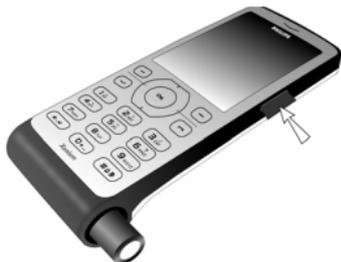
2. Press the card until it is locked in place.
