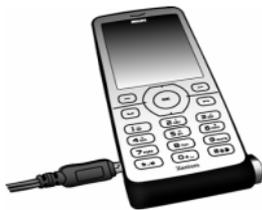
On the idle screen, the two battery symbols indicate the state of charging, the left one for the main battery and the right one for the AAA battery. During charging, the left indicator will scroll and it
