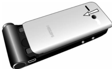
***When inserting the battery, be careful not to damage the metallic connectors of the SIM card slot.***
