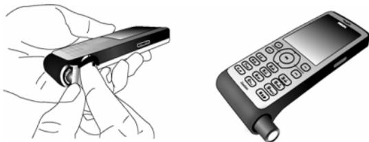
3. Tighten the battery cap by hand. Stop tightening the cap when it is secure (at the groove).
