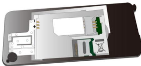
4. As shown, align the metallic connectors on the battery and battery slot. Insert the battery until it is locked.
