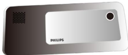
Remove the protective film covering the screen and camera lens before using the phone.
