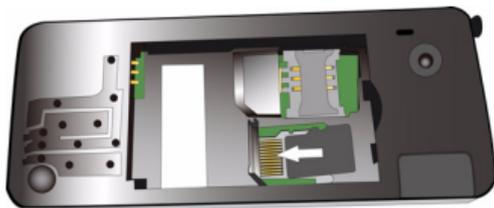
3. Press down the card holder and pull it until it is locked.
