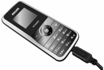
During charging, the charge indicators will scroll. It takes around 3 hours to fully charge the battery. When all the scroll bars are steady, the battery is
