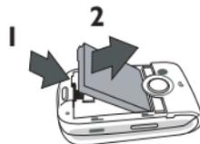
3. Remove the SIM card from its holder and slide it in its slot until it stops. Be careful that the connectors are facing downwards.
