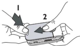
2. Remove the battery by lifting it with the grip as shown below.
