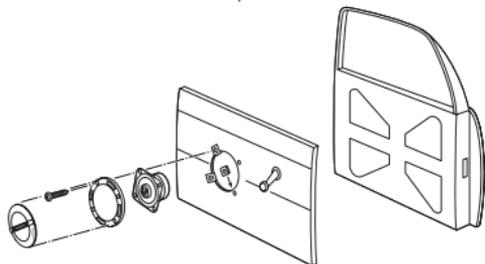
9 Press and insert the edges of the grille net.
