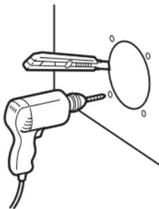
5 Cut out the marked area and drill the bolt holes.
