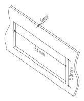
2 Install the sleeve into the dashboard and bend the tabs outward to fix the sleeve.
