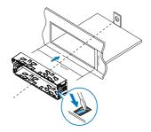
3 Place the supplied rubber cushion over the end of the mounting bolt.
