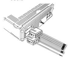
2 Check the car's wiring carefully and connect them to the supplied male connector.
