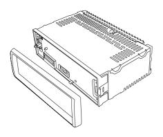
2 Insert the right side of the panel in the chassis until it is correctly engaged.
