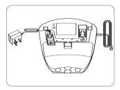
3 Connect the other end of the line cord to the telephone line socket and the other end of the power cable to the electricity socket.
