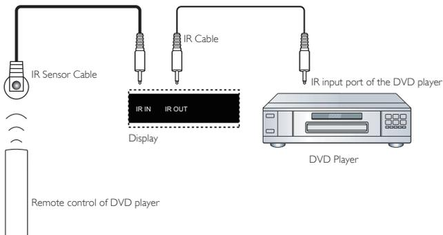
1. Connect the "IR Sensor Cable" to the [IR IN] port of the display.
