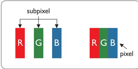
A pixel, or picture element, is composed of three sub-pixels in the primary colors of red, green and blue. Many pixels together form an image. When all sub-pixels of a pixel are lit, the three colored sub-pixels together appear as a single white pixel. When all are dark, the three colored sub-pixels together appear as a single black pixel. Other combinations of lit and dark sub-pixels appear as single pixels of other colors.
