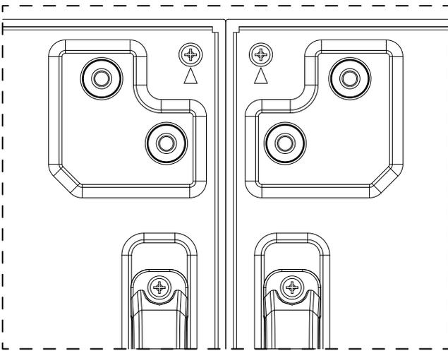
Install "Edge Alignment Kit-2" with 4 PCS of screw on outer, bigger holes.
