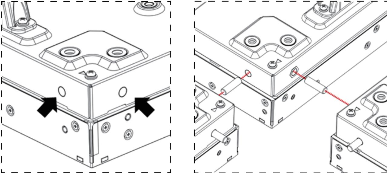
There are 8 holes on the four corners of displays designed for plug-in the edge alignment pin.
