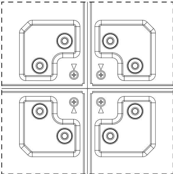
Install "Edge Alignment Kit-1" with 8 PCS of screw on outer, bigger holes.
