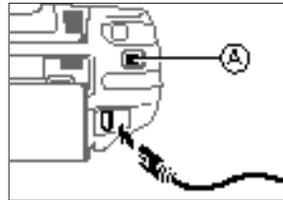
The battery supply will be switched off when the set is connected to the mains. To change over to battery supply, pull out the plug from the unit's AC MAINS socket.
