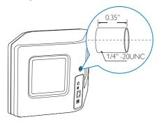
Through this hole, you can easily mount the device onto wall with a suitable mounting bracket. The mounting bracket is not included and you need to purchase one. Please follow the instructions included with your purchased wall mounting bracket.
