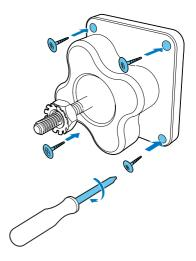
Insert the mounting screw on the bracket into the hole at the back of AW3000, then turn the rotating handle to tighten the screw.
