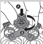
**7** Put the retaining frame back into the shaving unit (A) and turn the lock clockwise (B).
