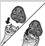
**8** Insert the lug of the new shaving unit into the slot in the top of the shaver. Then close the shaving unit.
