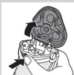
**3** Press the release button to open the shaving unit.
