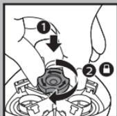
**5** Put the retaining frame back into the shaving unit (1) and turn the lock clockwise until it locks into place (2).
