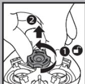
**3** Turn the lock counterclockwise (1) to unlock and remove the retaining frame (2).
