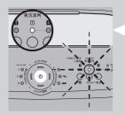
The filter cleaning light and the filter replacement lights indicate which filter has to be cleaned or replaced.
