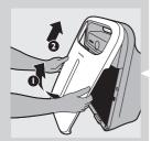
Tip: Place the appliance against a wall for more stability when you remove or insert filters.
