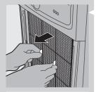
3 To remove filter 1 (pre-filter), grab the two projections and pull the filter towards you.
