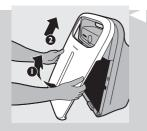
1 Place your fingers in the recesses of the side panels and gently pull the bottom of the front panel towards you. Then lift the hooks at the top of the panel out of the top of the appliance.
