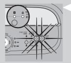
Note: When the power on/off light, filter replacement light 2 and the 'REPLACE FILTER' light are on continuously, the appliance is locked (see section 'Filter maintenance' in this chapter for more information).
