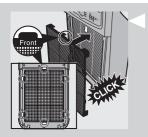
7 Put filter 1 (pre-filter) back into the appliance.
