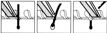
Groove channels beard closer to cutting system Lifter raises hair Blade cuts hair which then drops below skin level
