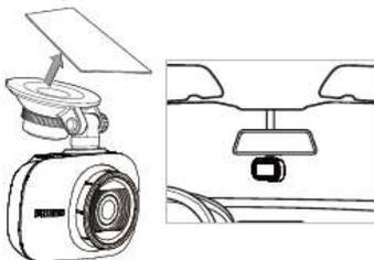
3. Adjust the position of the device within the mount to ensure you're recording a clear view of the road.
