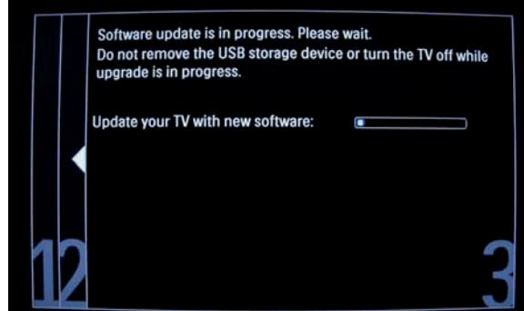
6. When the software upgrade is complete, remove the USB drive. Turn the set off and back on.
