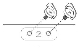
• Using "Edge Alignment Kit-2" on adjacent four displays.
