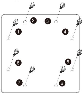
• Using "Edge Alignment Kit-2" on adjacent two displays.
