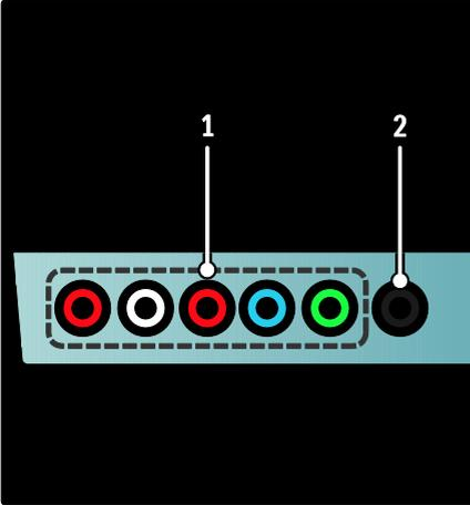
1. **CVI 1** (Audio L/R and YPbPr): Video input from analog devices such as DVD, receiver, game console, etc. This connector is used with audio input.
