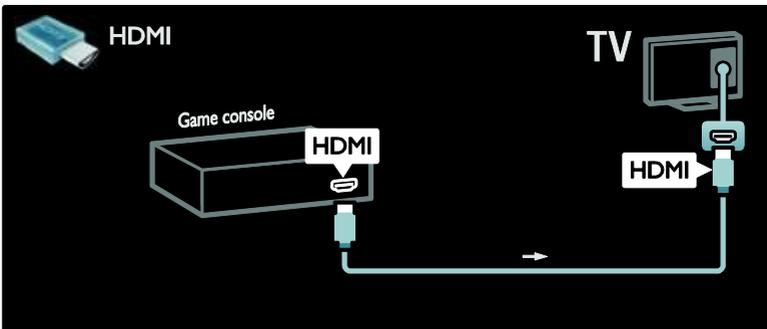
Otherwise, connect the game console to the HDMI or the EXT2 (YPbPr and Audio L/R cables) connectors on the bottom of the TV. (On certain models, EXT2 is labelled EXT3).
