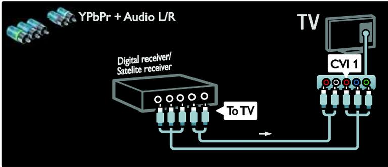
Finally, use two YPbPr cables to connect the two devices and the TV.
