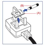
This apparatus is supplied with an approved moulded 13A plug. To change a fuse in this type of plug proceed as follows:
