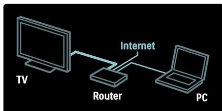
1. Switch on the router and switch on its DHCP setting.
