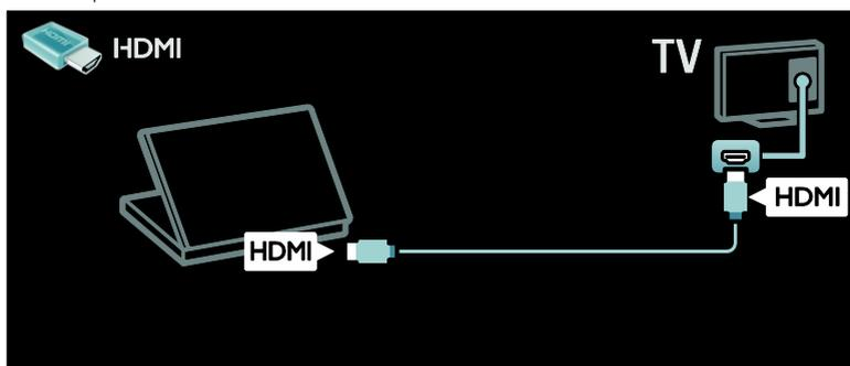
Connect the computer with a DVI-HDMI cable to the TV.
