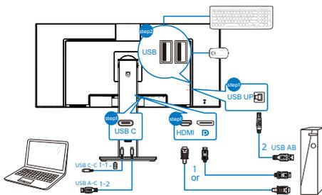
3. Enter to OSD menu. Go to KVM layer and select “Auto”, “USB C” or “USB up” to switch the control of peripherals from one device to another. Simply repeat this step for switching the control system using one set of peripheral.
