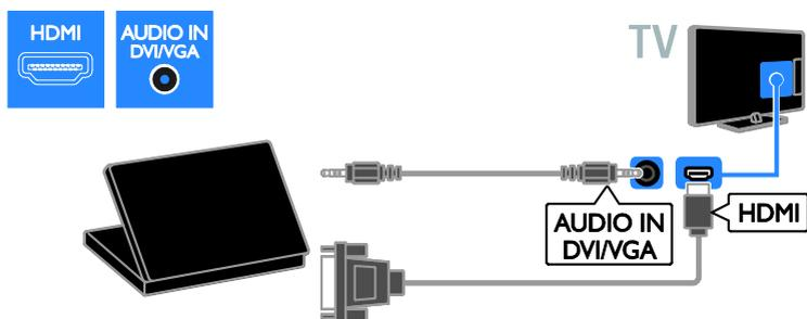
Connect the computer to the TV with a VGA cable and an audio cable.
