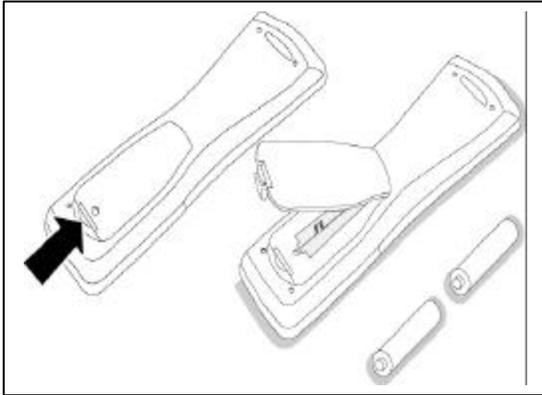
To load the supplied batteries into the remote control:
