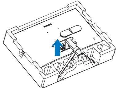
3. Use a screwdriver to remove the screws on the arm, and then detach the arm/stand from the monitor.
