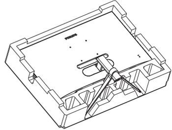
2. Remove the hinge cover from monitor body by using auxiliary tool.
