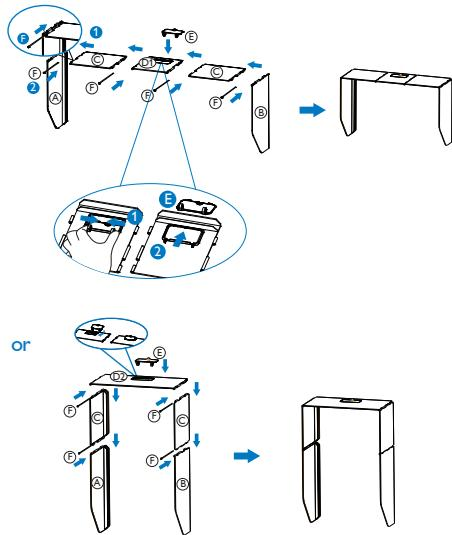
3. Slide down the shading hood on the top of the monitor.
