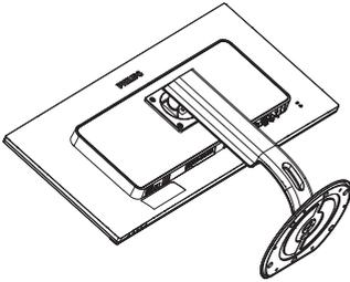
2. Loosen the assembly screws, then detach the neck from the monitor.
