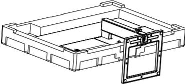
2. While keeping the release button pressed, tilt the stand and slide it out.
