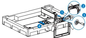
3. After attaching the base, erect the monitor with both hands on holding the monitor together with styrofoam firmly. Now you can pull out the styrofoam. When you pull out the styrofoam, do not squeeze the panel to avoid broken panel.
