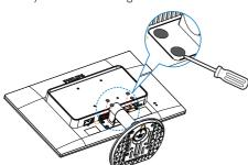
3. Remove the screws from hinge cover.
