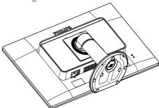
2. Remove the screws from hinge cover.
