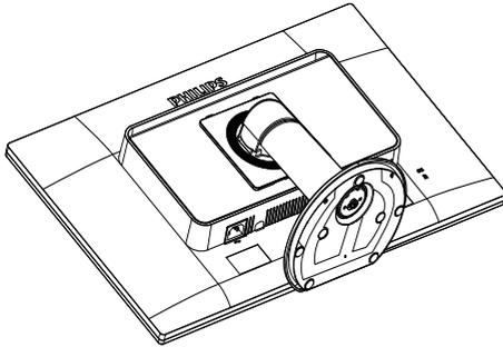
2. Remove the screws from hinge cover:
