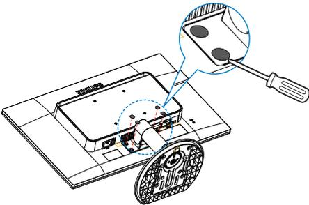
3. Remove the screws from hinge cover.
