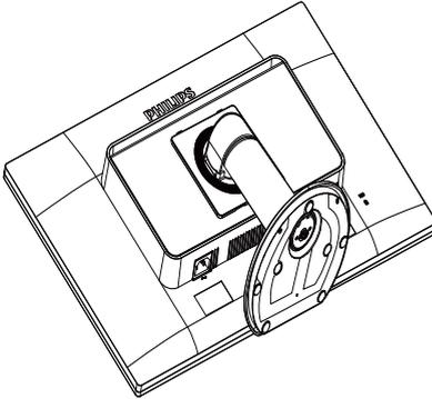
2. Remove the screws from hinge cover.
