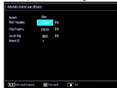
You can select frequency ranges from this screen. For highlighting lines you see, use ▲ or ▼ button. You can enter the frequency range manually by using the numeric buttons on the remote control. Set Start and Stop Frequency as desired by using numeric buttons on the remote control.
