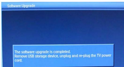
7. When the Software Upgrade Complete screen appears, unplug the TV from the AC outlet, remove the USB drive, then wait for 30 seconds before re-plugging.
