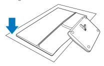
Hold the monitor and base with both hands. Gently bend the base vertically down to a fixed angle.
