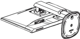
3. Loosen the assembly screws, then detach the neck from the monitor.
