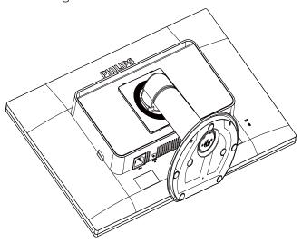
2. Remove the screws from hinge cover.
