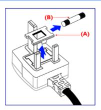
outlets, it should be cut off and an appropriate 3pin plug fitted in its place.
