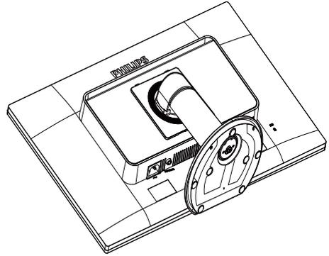
2. Remove the screws from hinge cover.
