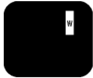
Three adjacent lit subpixels (one white pixel)
