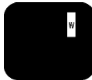
Three adjacent lit subpixels (one white pixel)
