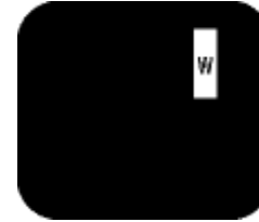
Three adjacent lit subpixels (one white pixel)
